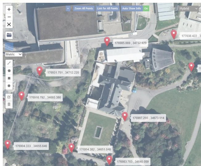
Figure 3: Locations of total coordinates in relation to traverse. [gridreferencefinder.com]
