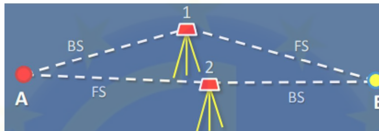
Figure 2: Shows a typical double set levelling position (Image courtesy of ELE)
